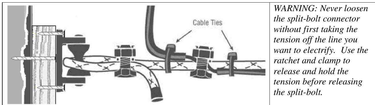
**WARNING:** Never loosen the split-bolt connector without first taking the tension off the line you want to electrify. Use the ratchet and clamp to release and hold the tension before releasing the split-bolt.
