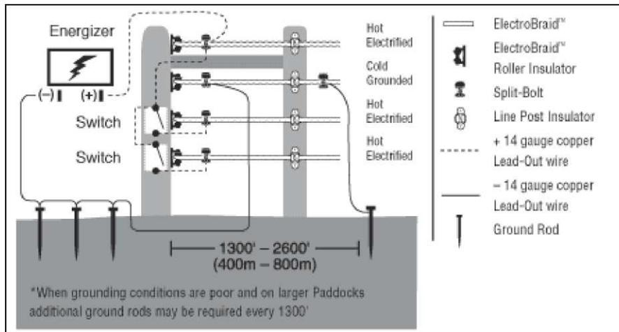
Heavy wet snow can short electric fencing. To prevent this, fences in areas prone to snow accumulation can be wired as illustrated above.
