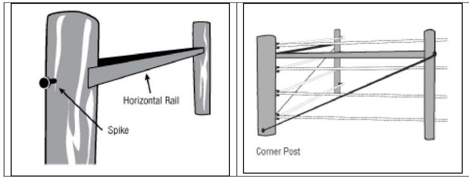
If your corner, end or gate post is large in diameter, you may want to pre-drill a hole for the spike through the post and into the end of the rail.
