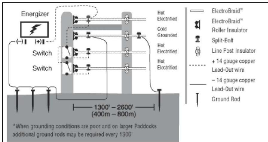
Heavy wet snow can short electric fencing. To prevent this, fences in areas prone to snow accumulation can be wired as illustrated above.
