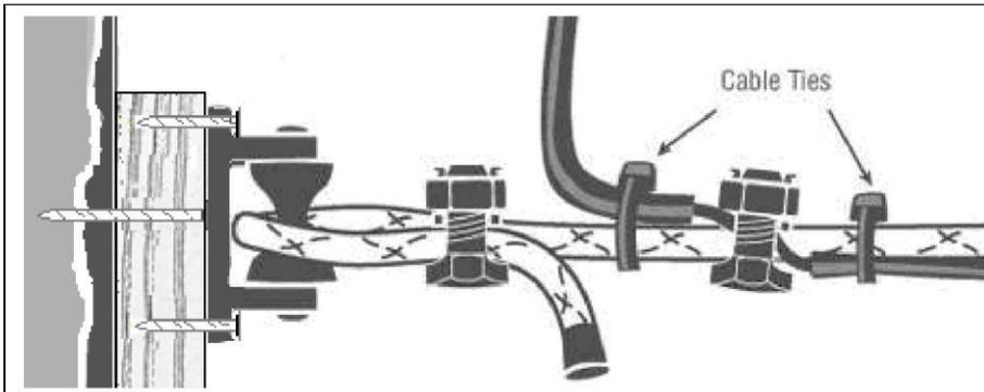
*WARNING: Never loosen the split-bolt connector without first taking the tension off the line you want to electrify. Use the ratchet and clamp to release and hold the tension before releasing the split-bolt.*
