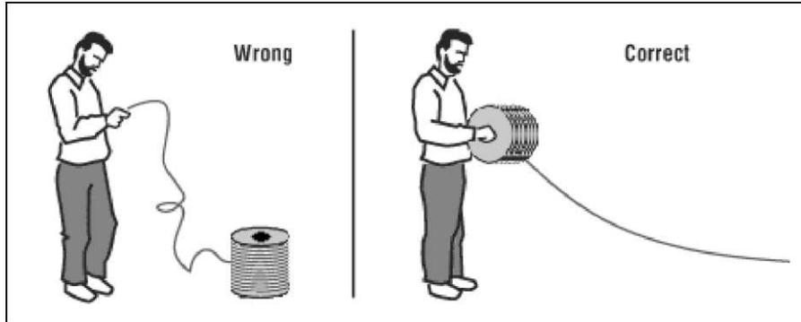
**DO NOT** take braid off one end of the spool. The Braid will kink and could be damaged. The correct method is to unroll the Braid and it will not kink. (see diagram)
