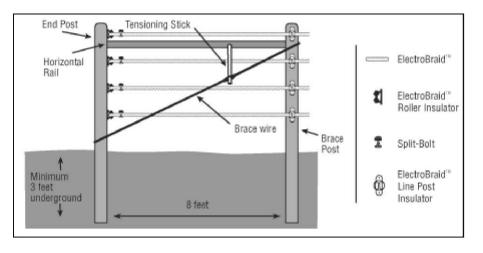
Whenever you fence a long, straight run you need to terminate and install a brace system every 2400 feet to maintain tension on the Braid<sup>TM</sup>.
