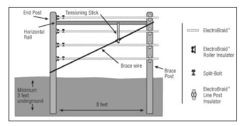
NOTE: To prevent an electrical short, make sure the brace wire and tensioning stick cannot contact any ElectroBraid<sup>TM</sup> strands
