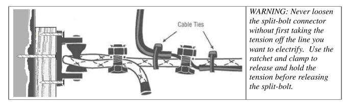
NOTE: For easier troubleshooting, it is best to use an extra Split Bolt Connector to connect your electrical components. If you want to disconnect the electrical from a strand you will not have to use the tensioning device to hold the tension.
